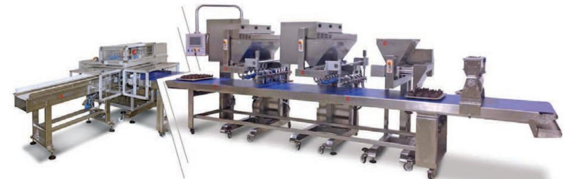
Designed to produce all sizes of muffins and cakes, plain or with filling of chocolate or fruit bites in the batter. The line operates on a continuous basis making it very fast and gentle. Units for adding various toppings including fatty crumbs are available. Also injecting system for chocolate, jam, and cream. Line is very easy to clean and operate.
