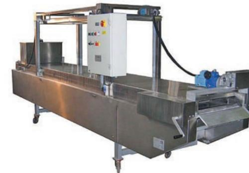
**WELLBAKE** offers state-of-the-art frying lines. Lengths of up to 7.5 meters, 600 to 1200mm in width.
